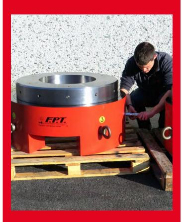
The hydraulic bolt tensioners with threaded insert are characterised by the threaded interchangeable insert which makes it possible to work on studs with various threads, using just one hydraulic cell.
