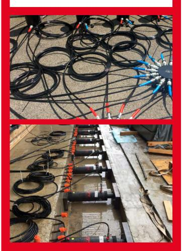
The 1000 bar thermoplastic flex hoses standard 1/4 version with internal Ø 6.3 mm are suitable for demanding applications and have a safety factor of 2.8: 1. On request, also available hoses with custom sizes and fittings, flexible hoses with internal Ø of 9.7 mm for applications with high flow rates as well.
